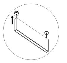
Raise the canopy and screw the knurled nut to keep the set in place.
